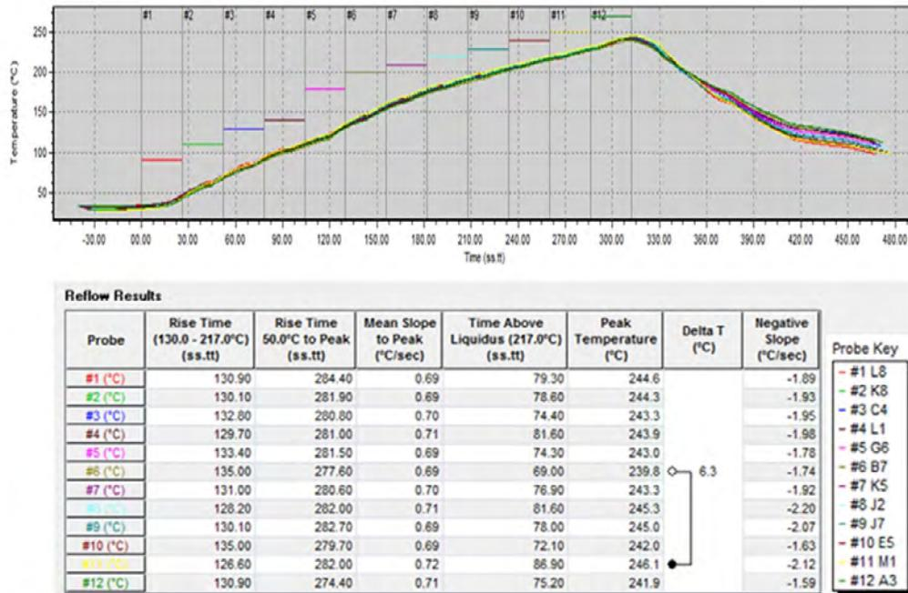
Figure 5: Reflow profile of a 93-mil board.
