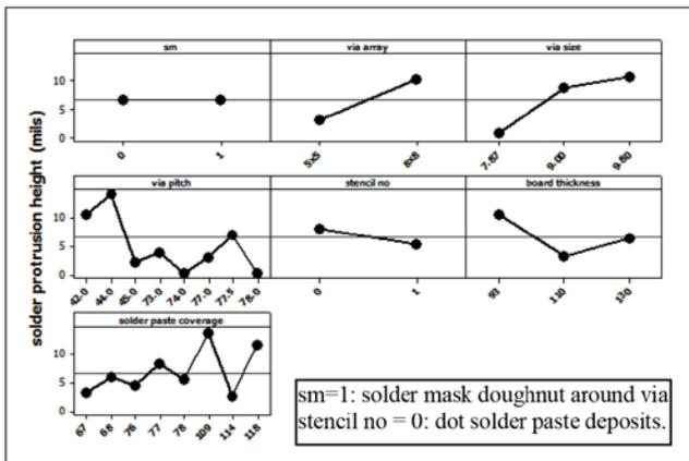
Figure 18: Main effects of solder mask (sm), via array, via size, via pitch, stencil type (dot=0, segmented=1), board thickness, and solder paste coverage on the solder paste protrusion height.
