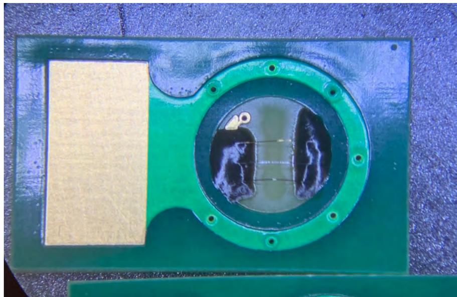
Figure 2: Glob top epoxy is used to encapsulate and protect bare dies.
