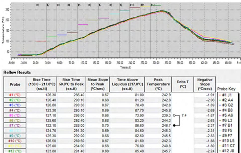
Figure 6: Reflow profile of a 110-mil board.
