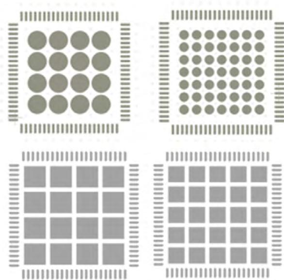
Figure 4: Dot and segmented apertures example.
