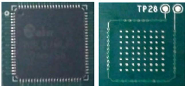
Figure 2: A-MLF88-10 mm-0.4mm -Sn, top and bottom side view on the board.
