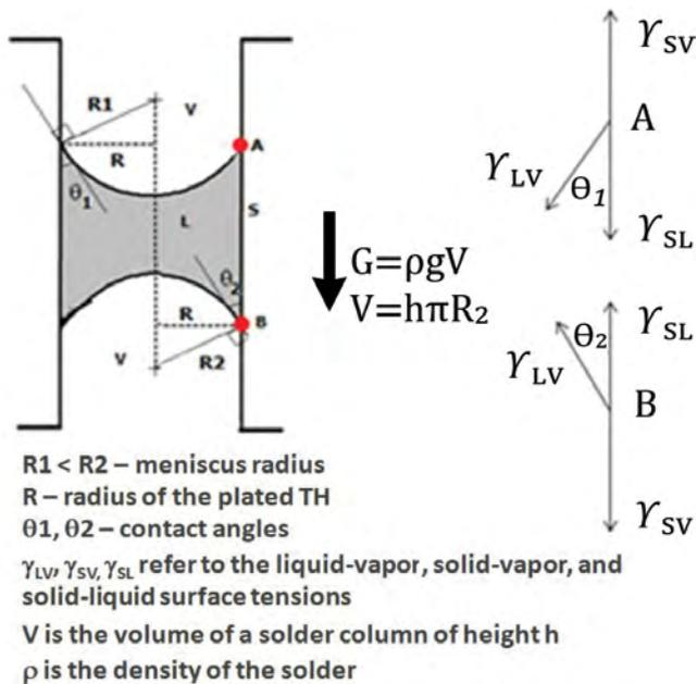
Figure 1: Equilibrium of forces acting on a finite volume of solder inside an exposed via.
