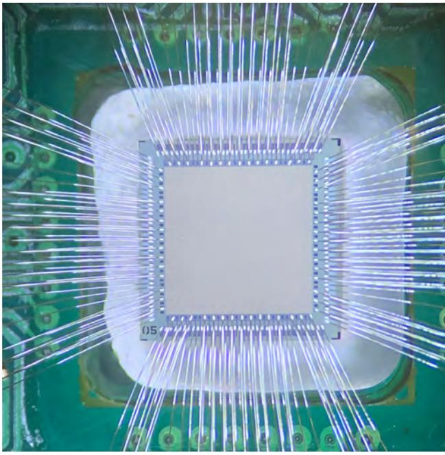
Figure 1: Stacked wire bonding is more complex than regular wire bonding and requires extra precision.
