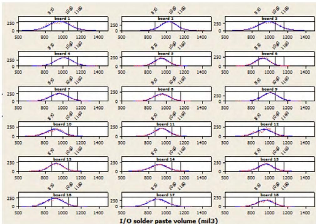
Figure 8: I/O solder paste volume by board.
