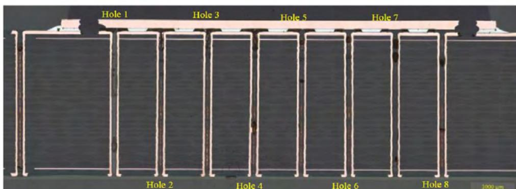
Figure 26: Cross-section at reference designator A7 ( $\phi 1 = 0.2$  mm  $\sim 0.00787$ "), PCA#18 (130-mil thickness).
