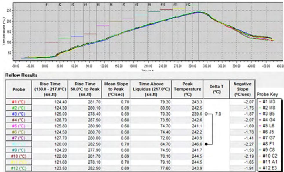
Figure 7: Reflow profile of a 130-mil board.
