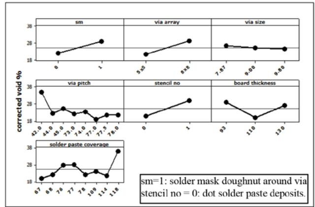
Figure 14: Main effects of solder mask (sm), via array, via size, via pitch, stencil type (dot=0, segmented=1), board thickness, and solder paste coverage on the corrected void% means.
