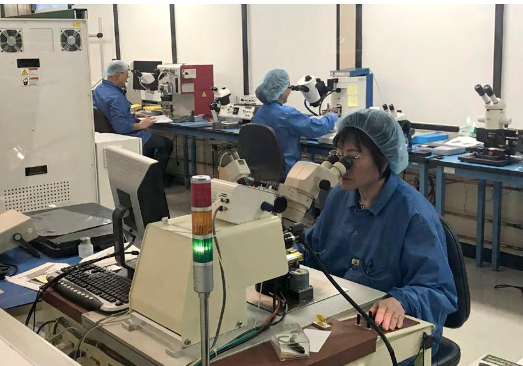
Figure 3: A Class 100 or 1,000 cleanroom is necessary for effective PCB microelectronics assembly.
