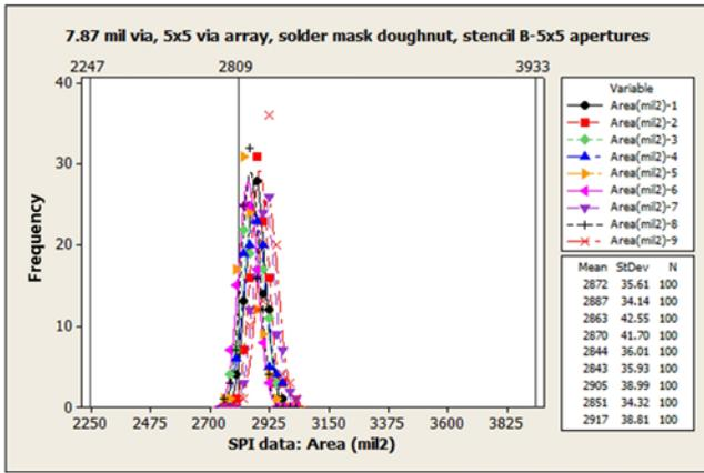
Figure 13: Thermal pad solder paste area–Stencil B.
